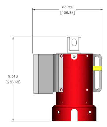
Lower adapter diameter will change and is dependent on valve bonnet size
